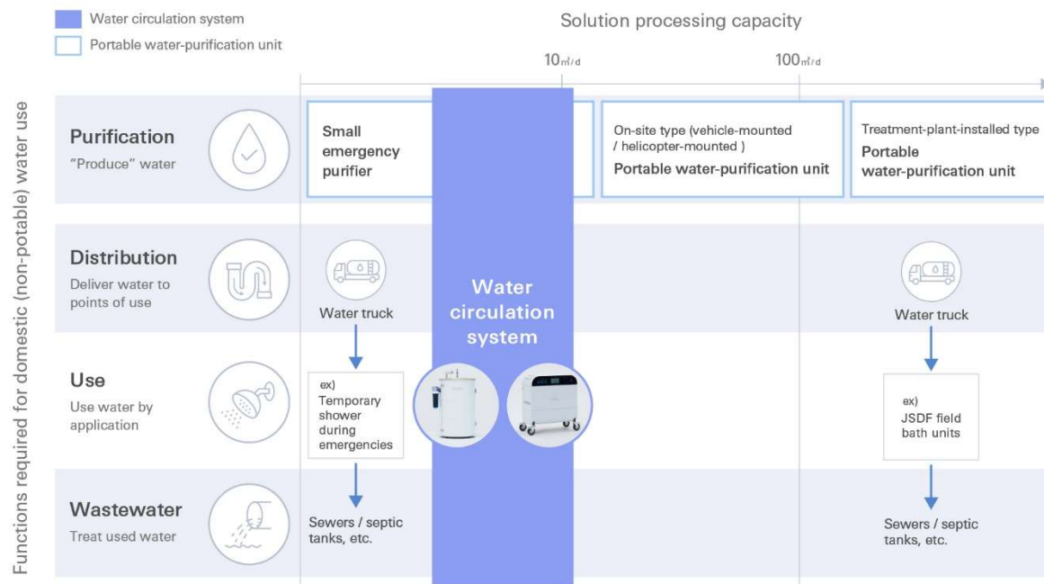
Figure 2. Functions of the Water Circulation System and Portable Water Purification Unit
